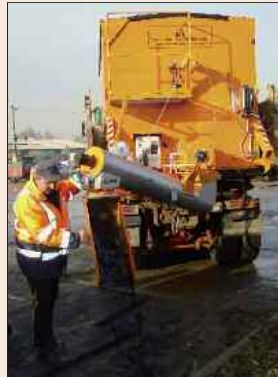
▶ ATC 100S with external worm conveyor
